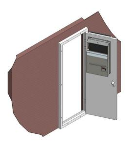
4. Fit the cover and fix it with the corresponding screws 4 x 50, 2 at the top and 2 at the bottom of the cover, tightening them in moderate way.
